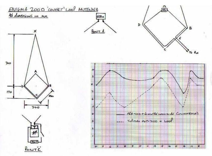
Take a 2metre length of ribbon cable and remove all but four conductors. This length is folded in half producing a 1metre length, the apex is point 'X'.
