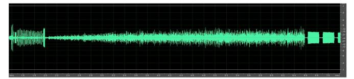
Examination of a number of these data bursts has shown that they are not identical & that there are variations in the length of some pulses as well as with the number of pulses sent.
