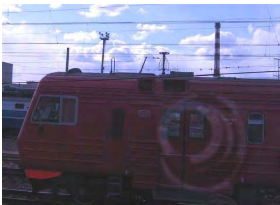
Airport train -- note folded dipole and discone in addition to long wire
