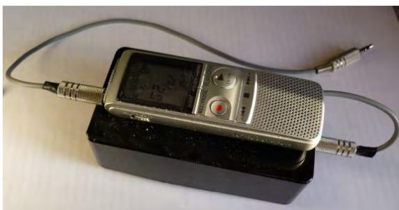
Battery box below the recorder holds two D Cells.
