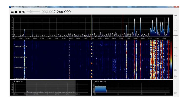
E07a 2040z 17/06 172 1 68076 8198 69 01802 ... 54334 000 000 Very strong signal received using the popular RTL-SDR TV dongle preceded by an HF upvertor and LF filter
