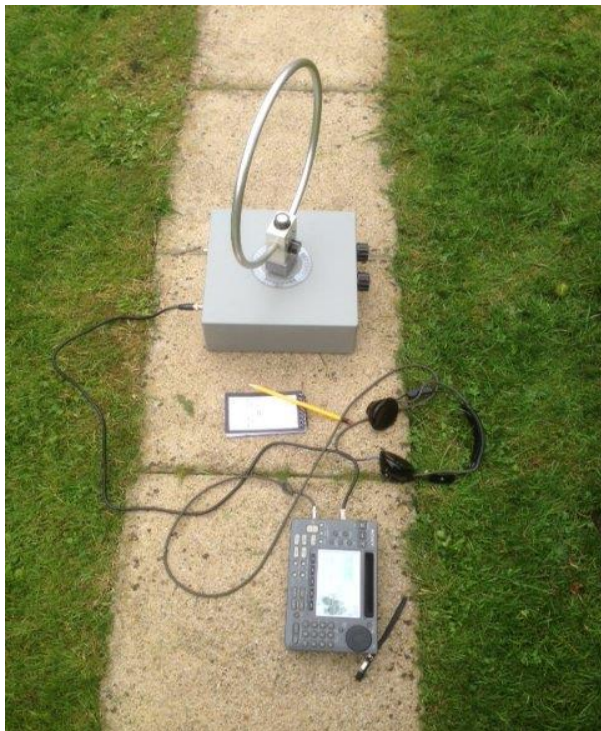
PLDn's RDF set-up with Sony ICF-SW55 & Homebrew RDF Unit
